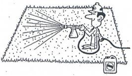
A hose sprayer which uses water pressure to draw chemicals, like weed killer, into a stream of water or a hose submerged in a bucket, pool or sink.
